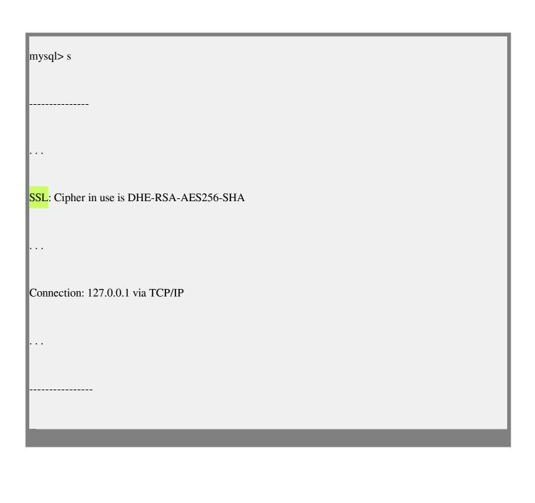
SSL cipher is displayed, indicating that SSL is being used to secure our connection.
