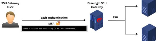
1. Edit the gateway user and enable "**Prompt Reason**." When the user SSH to ezsh, after the two-factor authentication step, the **shell will prompt them to enter a reason for the SSH** connection, which can be found under **shell activity**.
