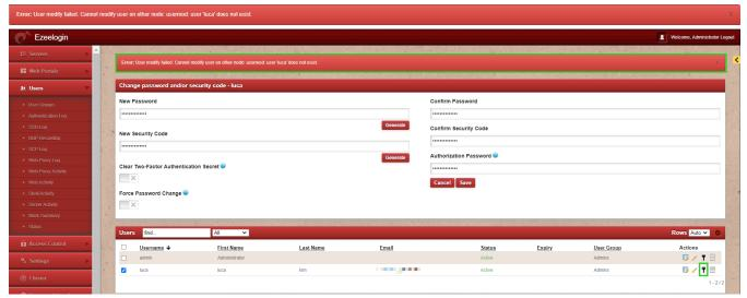
**Cause:** The error occurs when trying to modify a gateway user from the GUI (Master node) without the user being present on the Slave node (Secondary node). The system requires the user to exist on both nodes to apply modifications correctly.
